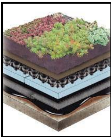
Figure 5: Extensive Green Roof, American Hydrotech
