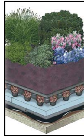
Figure 6: Intensive Green Roof, American Hydrotech
